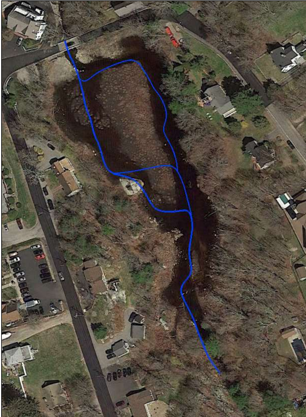
Figure A - Anticipated flow paths (blue) compared with post-removal conditions (aerial taken 4/22/2018). The primary flow-path is the eastern-most alignment.
